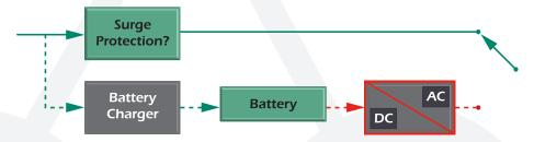
System performance is verified under only two conditions: 1) if / when it is periodically tested, and 2) during an emergency. MAY NOT provide surge protection, and DOES NOT provide power conditioning or regulated voltage to LED drivers and electronic ballasts that are being utilized for egress lighting. Inverters promoting 98+ % efficiency are off-line or standby designs, or "operating" in a bypass / standby mode.
