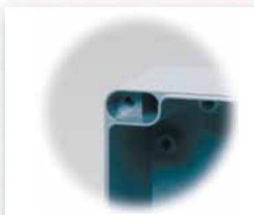
Wall mounting holes outside gasket area: maintaining water tight seal
